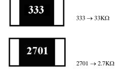
4. 4 Standard E-96 series values of 0603 ≤1% : due to the small size of the resistor's body, 3 digits marking will be used to indicate the accurate resistance value by using the following multiplier & resistance code. Multiplier Code (for 0603 ≤±1% marking)
