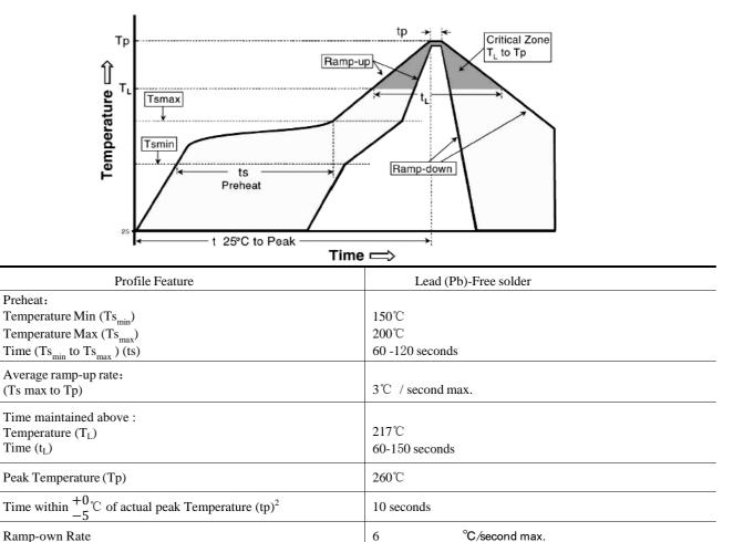
Time 25°C to Peak Temperature Allowed Re-flow times : 2 times
